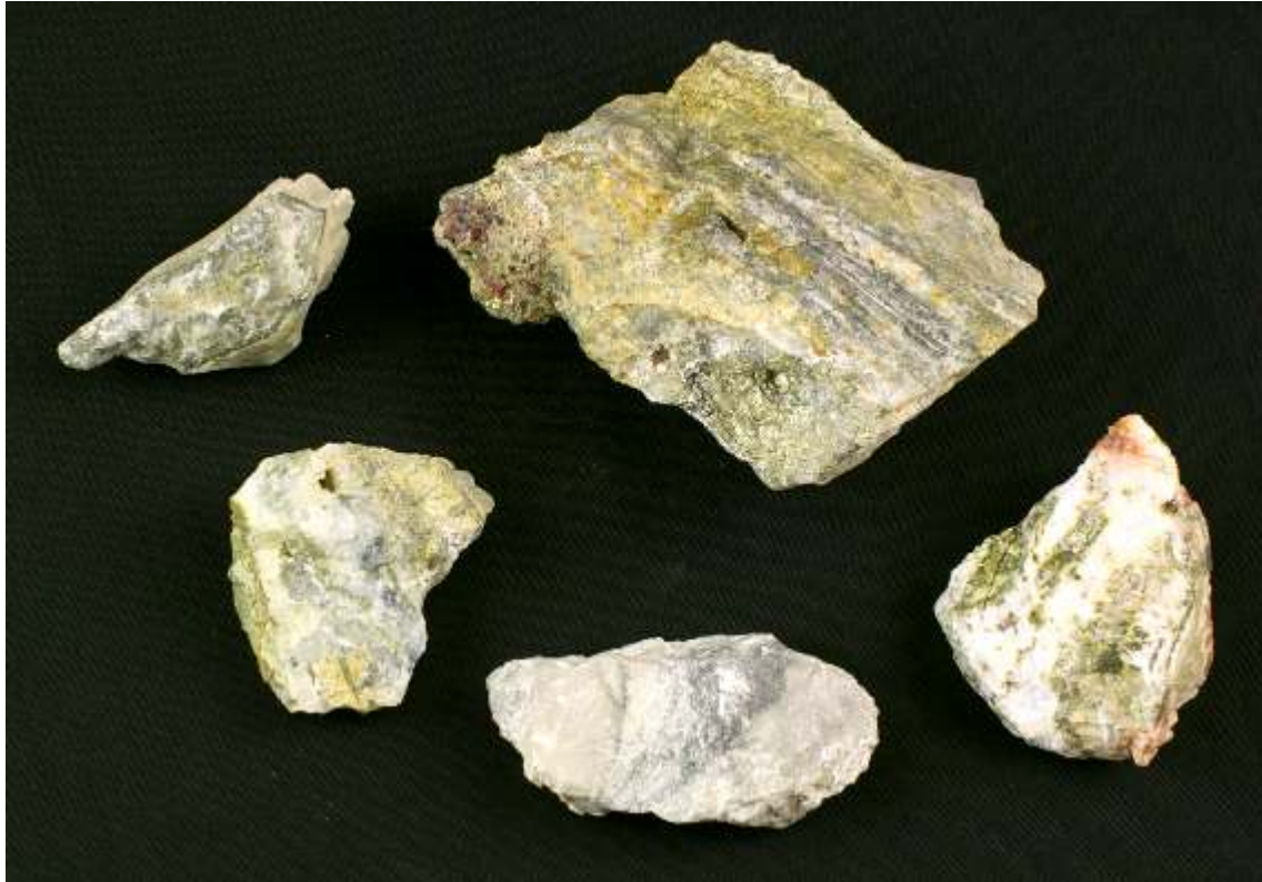
Telluride gold in the form of petzite (the dark mineral in this picture) in quartz
